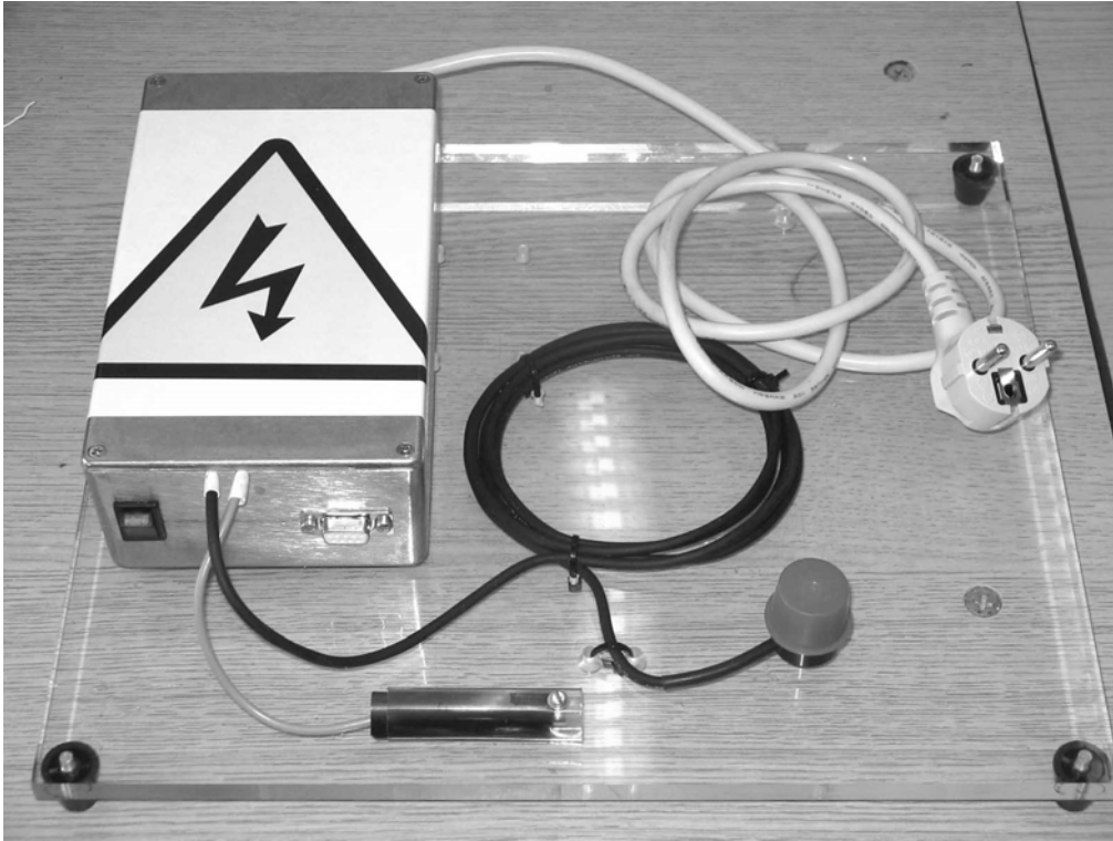
Fig.5 Data acquisition system with flash memory and battery for emergency power supply, RS232 interface
